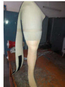
HITECH PROSTHESIS with four bar linkage Knee Joint with HITECH Foot
